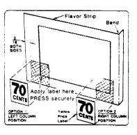
In the MPC vender the price labels are fastened to the flavor cards before the flavor cards are inserted into the selection buttons. To insert the flavor cards into the selection buttons swing the coin changer mounting plate away from the outer door exposing the back of the selection buttons. The flavor cards can be inserted into the back of the selection buttons from either side. Ensure that the flavor cards are placed in the selection buttons that correspond to the columns the product is in.
