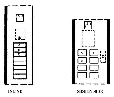
When the Service mode is entered the vender starts with the Group 1 accounting functions. The 3 accounting functions will repeat with successive pushes of select buttons A + B. If the Group 2 setup functions are entered the 4 set-up functions will repeat with successive pushes of select buttons A + B. The following shows the different displays and explains the different modes.
